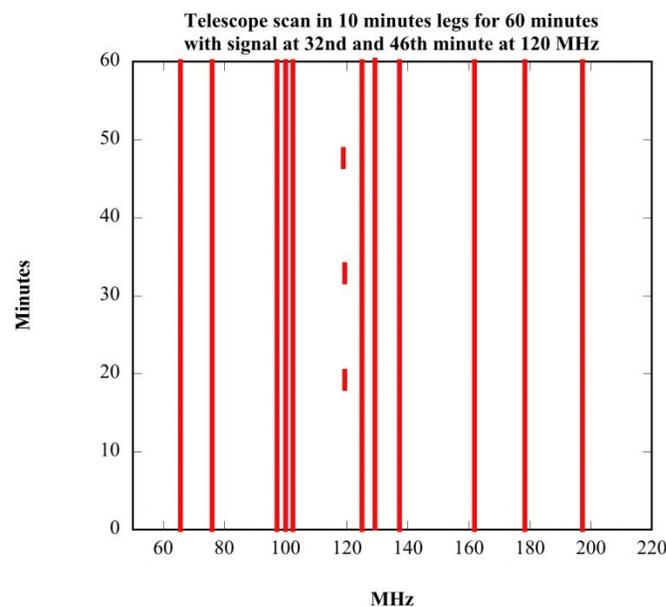
They are a graph that shows an x-y plot with the frequency of light plotted on the x-axis and time plotted on the y-axis. Data from the radio telescope's scans are compiled into these graphs which in turn help us separate signals from interference. A real signal will only last for a short period, while the longer signal, which is interference, will always be there. The signals that may be of extraterrestrial origin will disappear when radio telescope points in another direction.
